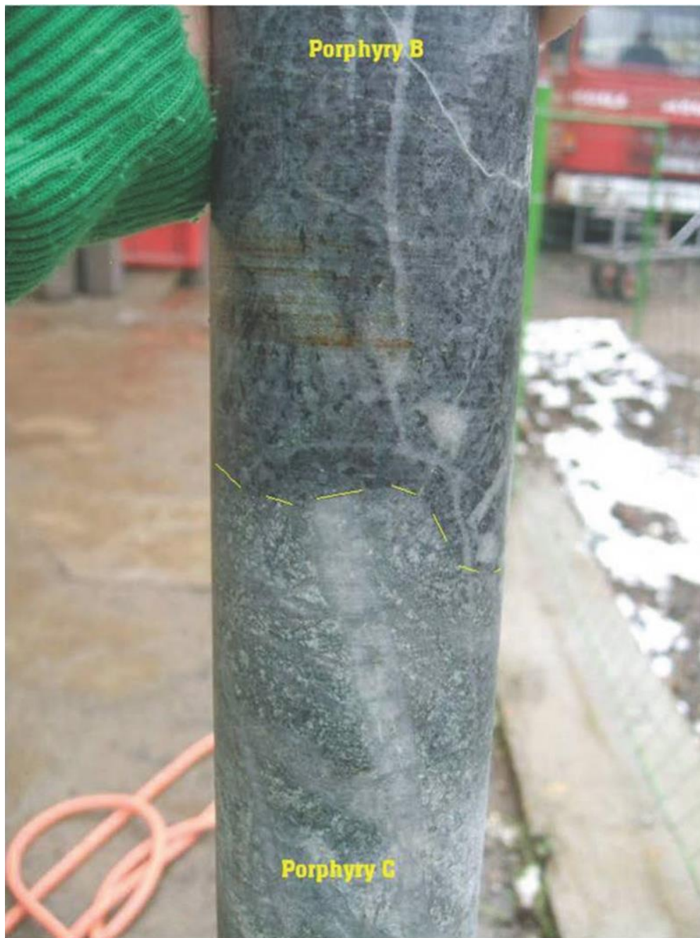
Figure 7.9: Photograph of Drill Core from RRD-45 Contact between Porphyry C and Porphyry B
