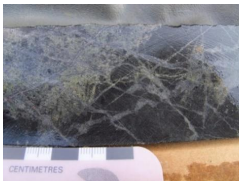
Inter-Mineral Porphyry and Sediment Contact in Hole RGD-17 at 454 m
